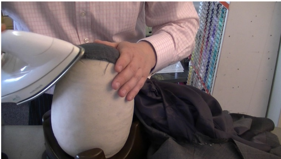
The standard tailors ham cradled in the ham holder pressing a sleeve head.
