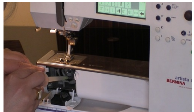
Oiling the bobbin race
