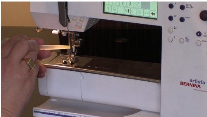
Oiling the sewing machine needle clamp mechanism
