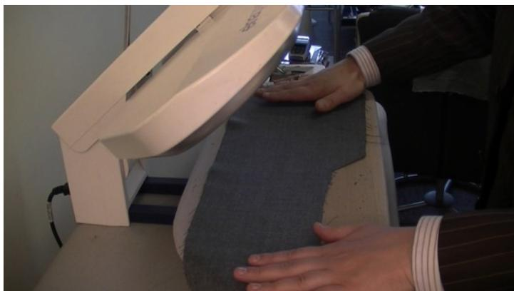
Getting the fabric panels ready on the press before the interfacing will be bonded to the cloth.
